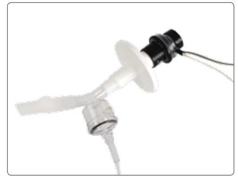
Integrated dosimeter for automatic broncho-challenge tests
