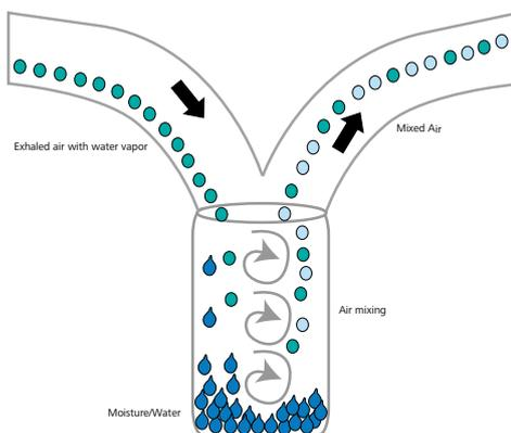
Moisture must be removed from the sample tubing to achieve accurate measurements and to prevent contamination and damage to the device. Conventional water traps introduced additional problems when used to remove excessive moisture:
